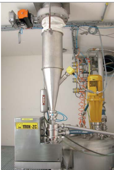
YTRON-ZC with powder addition via silo Application: Suspending of Spices
